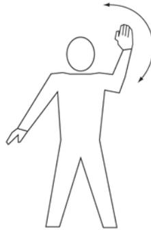
Point right arm downward, left arm repeatedly moved upward-backward. Speed of arm movement indicating rate of turn. **TURN TO THE LEFT**
