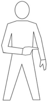
Right or left arm down, other arm moved across the body and extended to indicate direction of next marshaller. **PROCEED TO NEXT MARSHALLER**
