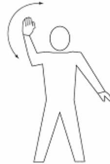
Point left arm downward, right arm repeatedly moved upward-backward. Speed of arm movement indicating rate of turn. **TURN TO THE RIGHT**
